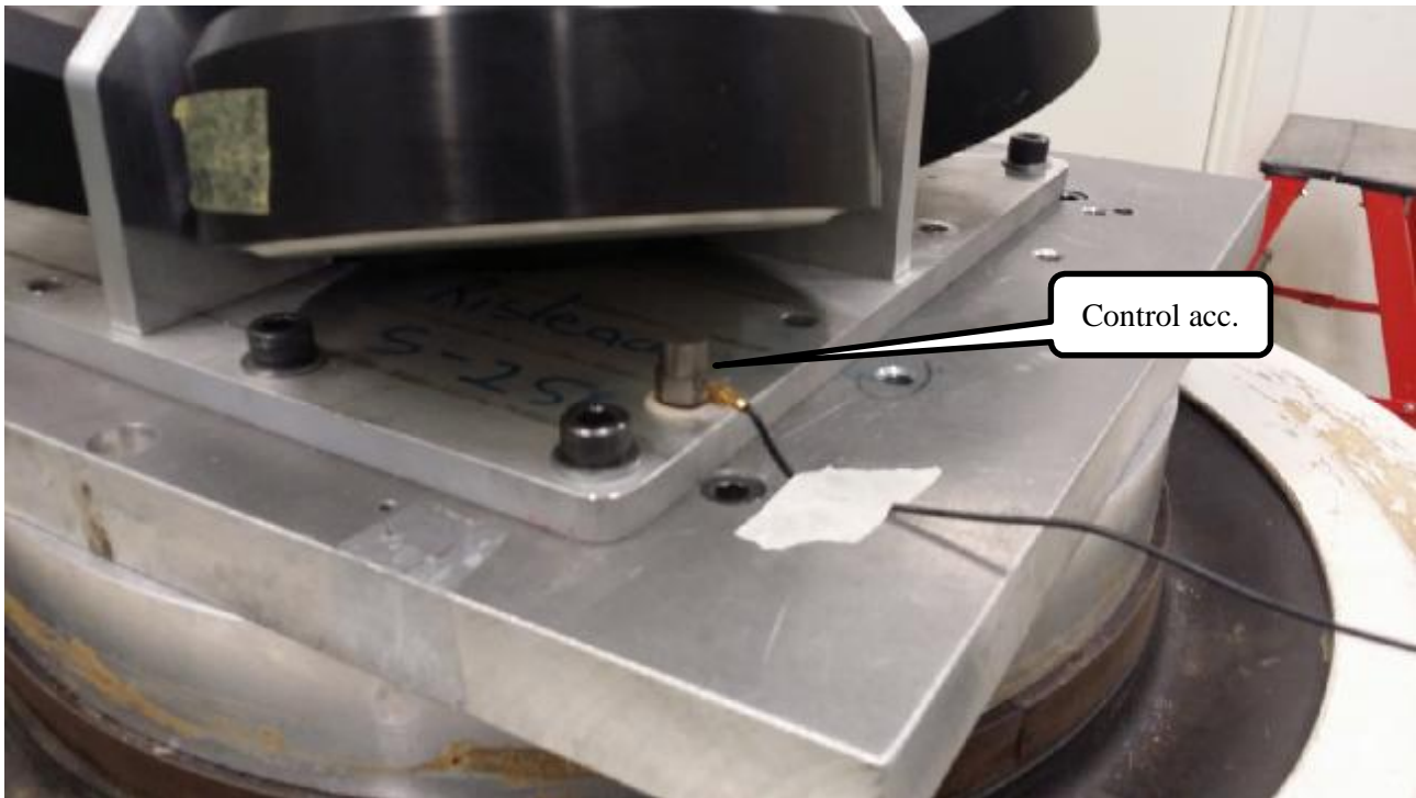
Figure 9 - Control accelerometer in Z-axis
