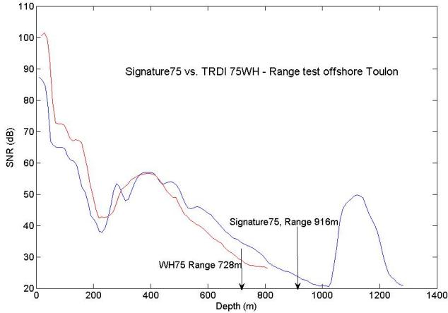
**Figure 4 - Comparing the amplitude data from a Signature75 and a WH 75 kHz, both operating with 10m cells and in narrowband mode (about 6% bandwidth)**
