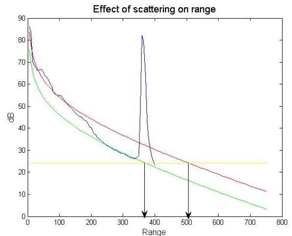
Figure 2 - Scattering from the ocean (blue), decay level fitted to the upper portions of the water column (red) and the lower part of the water column (green).
