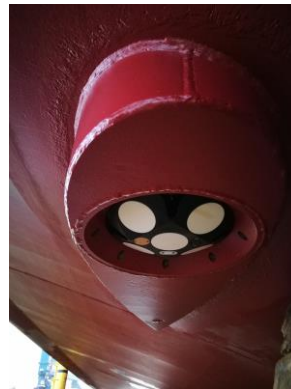
Figure 2 and 3: A NORTEK Aquadopp Profiler mounted in a TRIAXYS™ with Currents Buoy (left) The NORTEK Signature500 VM hull mounted on the vessel Geo Focus (right)
