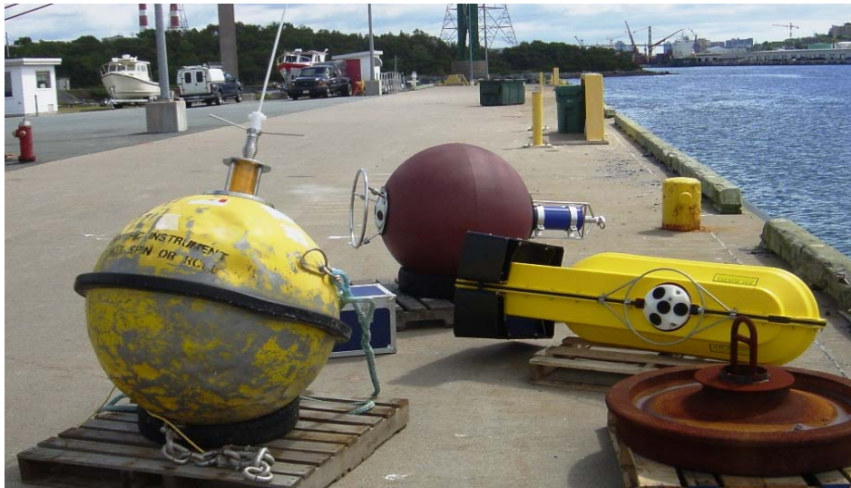
Fig.2 Test equipment (left to right): Datawell Waverider (DWR), AWAC in Sphere buoy with battery canister below, AWAC in SUBS buoy.
