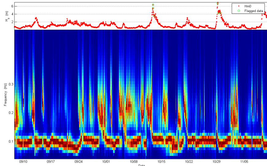
Fig. 11 Normalized energy spectrogram for the velocity measurements from the Sphere with H_s provided on top for reference.
