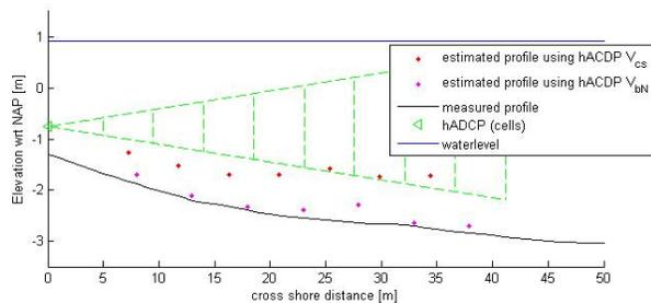
Figure 10. Depth profile reconstructed from 800 s timeseries on Tuesday June 8<sup>th</sup> around 12:12. Black line represents the profile as measured using the jetski. Red points are depth estimates from cross correlation of the cross shore velocity signals of the hADCP, magenta points are depth estimates using the northern beam velocity signals.
