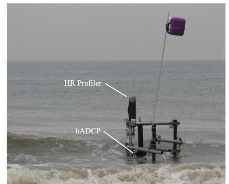
Figure 3. Measurement frame on Tuesday June 8<sup>th</sup>. The purple can serves as a buoy, mounted slightly outside the beams of the HR profiler.
