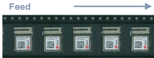
Figure 13: Orientation of NINA-B112 modules on tape
