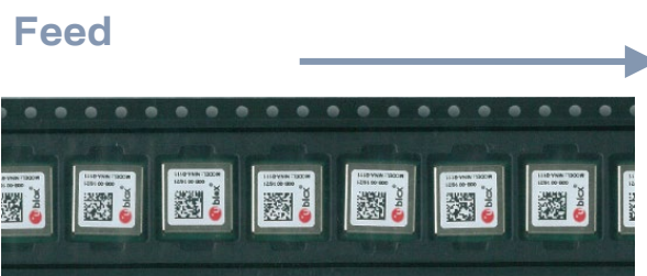
Figure 12: Orientation of NINA-B111 modules on tape
