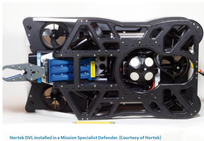
Nortek DVL installed in a Mission Specialist Defender. (Courtesy of Nortek)
