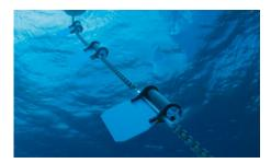
The Aquadopp 300 m is a compact, accurate and affordable single-point current meter for applications where a current profile is not needed. Designed for use in a number of deployment scenarios from mooring lines to bottom-mounted structures, it comes with PUV-based directional wave measurement capability as standard, making it the best value in the industry.
