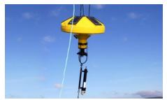
The Aquadopp Profiler is a highly versatile acoustic Doppler current profiler (ADCP) available in four profiling range options, from < 1 m to > 85 m. Designed for simple yet powerful operation, this current profiler is packed with features used by engineers and researchers to enable accurate and effective hydrodynamic data collection in a variety of environmental conditions.
