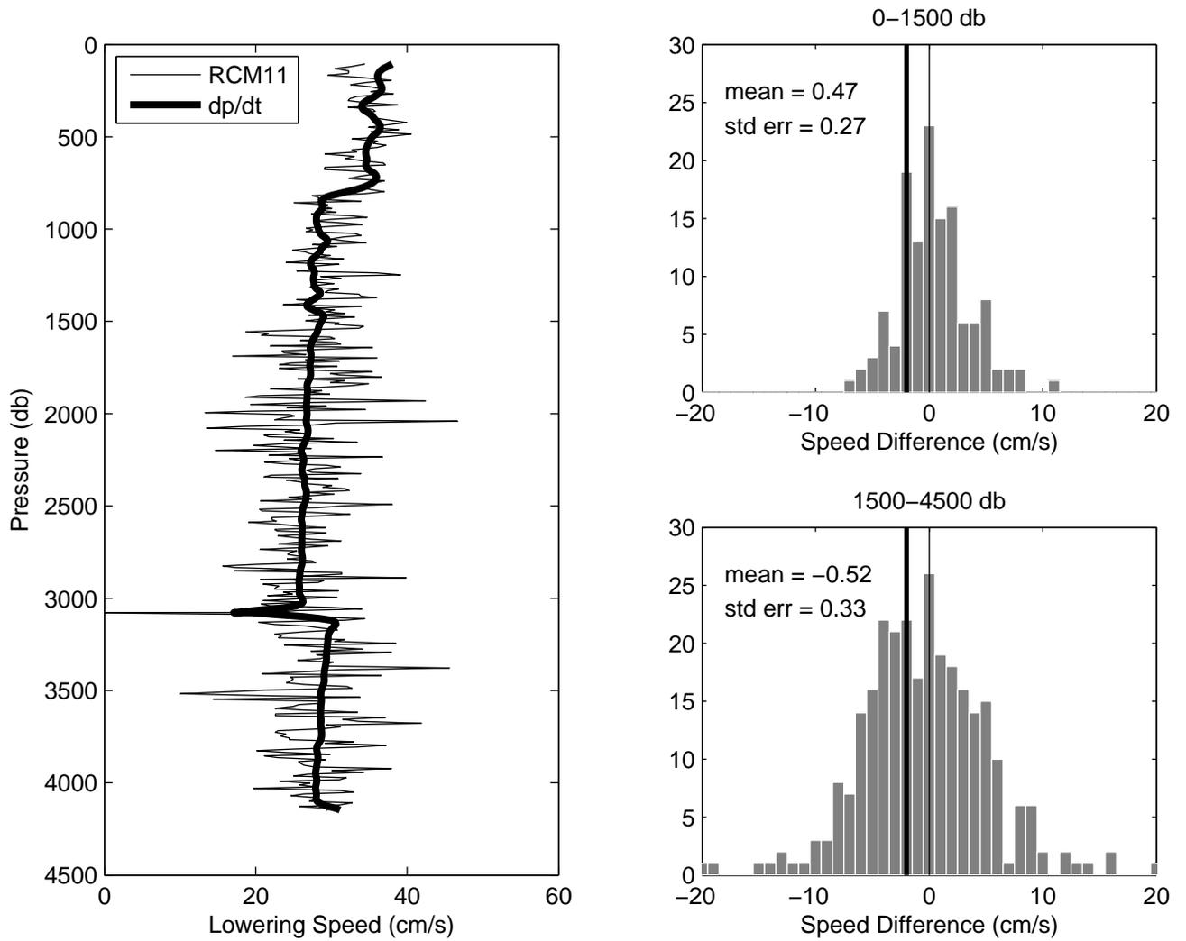
Figure 10: A comparison of the RCM11 vertical velocity with actual lowering speed for the second lowering test. The left panel shows the vertical component of the RCM11 velocity (thin noisy curve) and the lowpassed lowering speed (heavy smooth curve). The right hand panels contain histograms of the difference between the RCM11 vertical velocity and that calculated in two pressure intervals. The fine vertical line is at -2 cm/s; the heavy one is at the origin.
