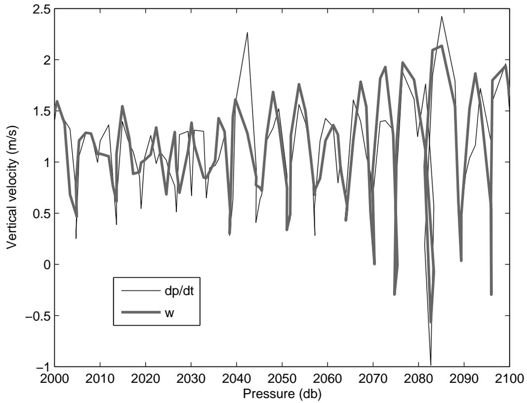
Figure 7: Vertical velocity computed from the rate of change of pressure and from the Doppler shift of acoustic signals as measured by a 3rd generation AQD.
