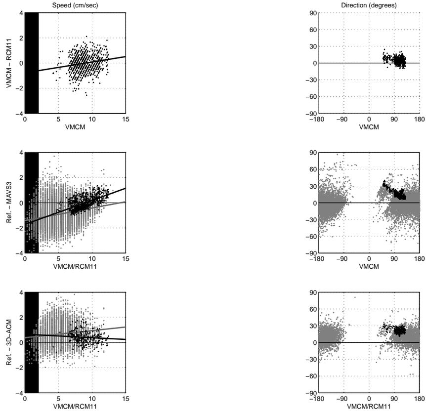
Figure 5: As in Fig. 2, but for the Minimoor deployment, that contained a VMCM rather than a VACM. Because the VMCM failed after two days we have used two means of comparison: the dark black points and lines are derived from differences with the VMCM for the first two days and, for the lighter grey points and lines the RCM11. All RCM11 speeds have been adjusted by the factor  $9/8$  (see text).
