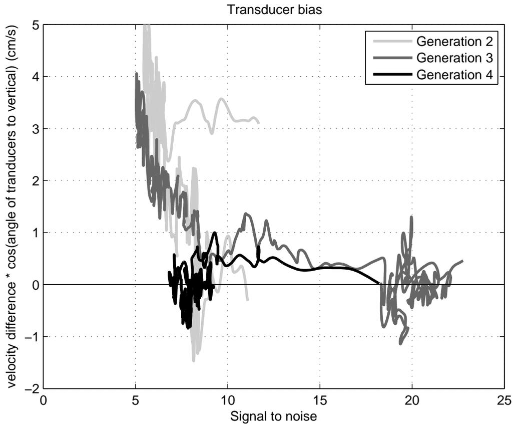
Figure 12: Transducer bias versus signal-to-noise for three generations of the AQD. The bias is calculated as the difference between the measured vertical velocity and the lowering rate projected into the relevant beam coordinate. The signal-to-noise is calculated as  $0.4 * (\text{signal strength} - \text{signal strength just after instrument recovery})$  according to the manufacturer's instructions (Atle Lohmann, pers. comm.).
