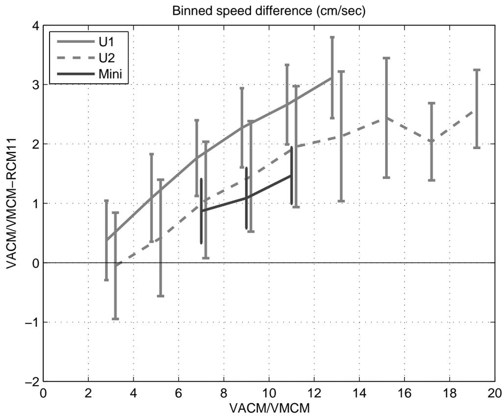
Figure 6: Binned differences between speeds measured by either a VACM or a VMCM and an RCM-11.
