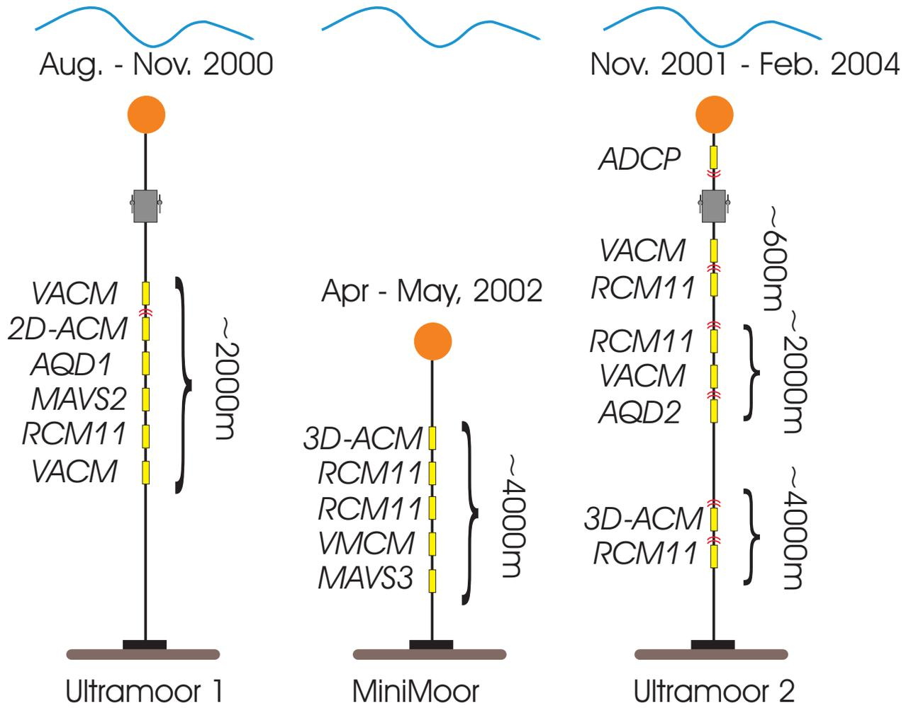
Figure 1: The 3 moorings on which current meters were compared.
