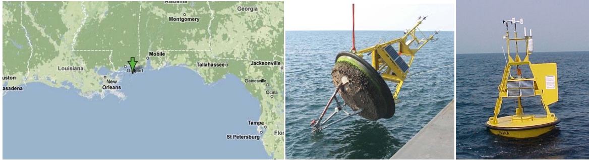
Fig. 2 Map of NDBC Station 42007 location (green arrow) in Gulf of Mexico and photos of 3 m disc buoy with bridal.
