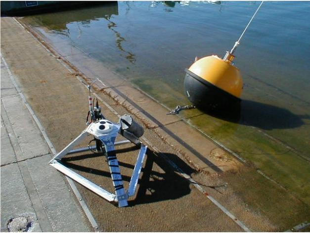
Fig. 3 Waverider and AWAC (center of triangular frame) prior to deployment.
