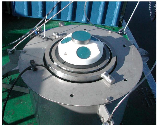
Fig. 11 The 600 kHz AWAC with enlarged center transducer.
