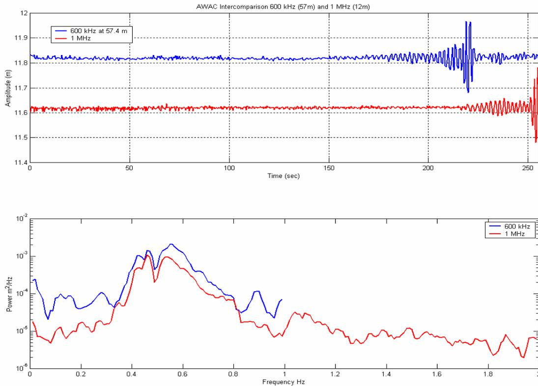
Fig. 12 Wave measurements for the 600 kHz (blue) and 1 MHz (red) AWACs. The top pane is the time series of the AST where the 600 kHz has been shifted from 57.4 meters to 11.8 meters for comparison purposes. The bottom pane shows the spectra for the two instruments, note the energy in these spectra would correspond to waves with a significant height of less than 10 cm.
