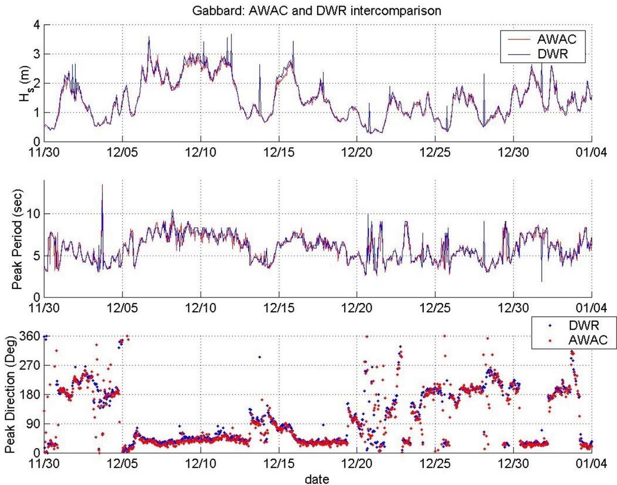
Fig. 4 Comparison results for the AWAC (red) and the Directional WaveRider (blue). Estimates provided in the three plots are significant wave height, peak period, and peak wave direction.
