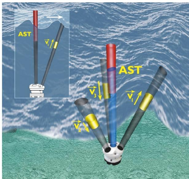
Fig. 1 Deployed AWAC with four beams
