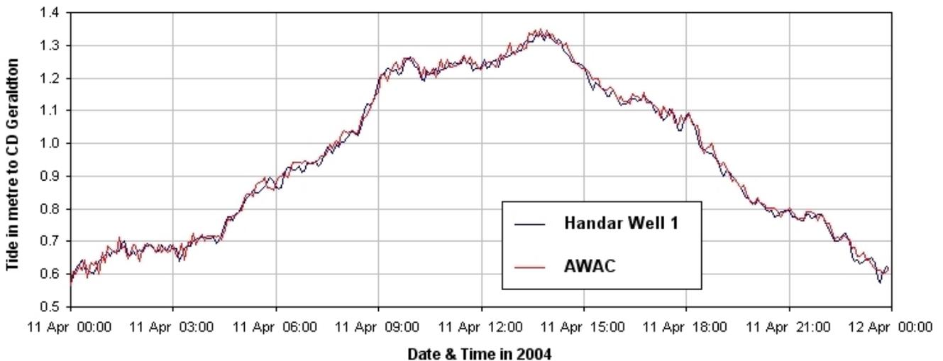
Fig.10 Comparison of water level estimates from the AWAC-AST and Handar tide recorder Geraldton, Australia. The analysis is compliments of MetOcean Engineering and Tremarfon
