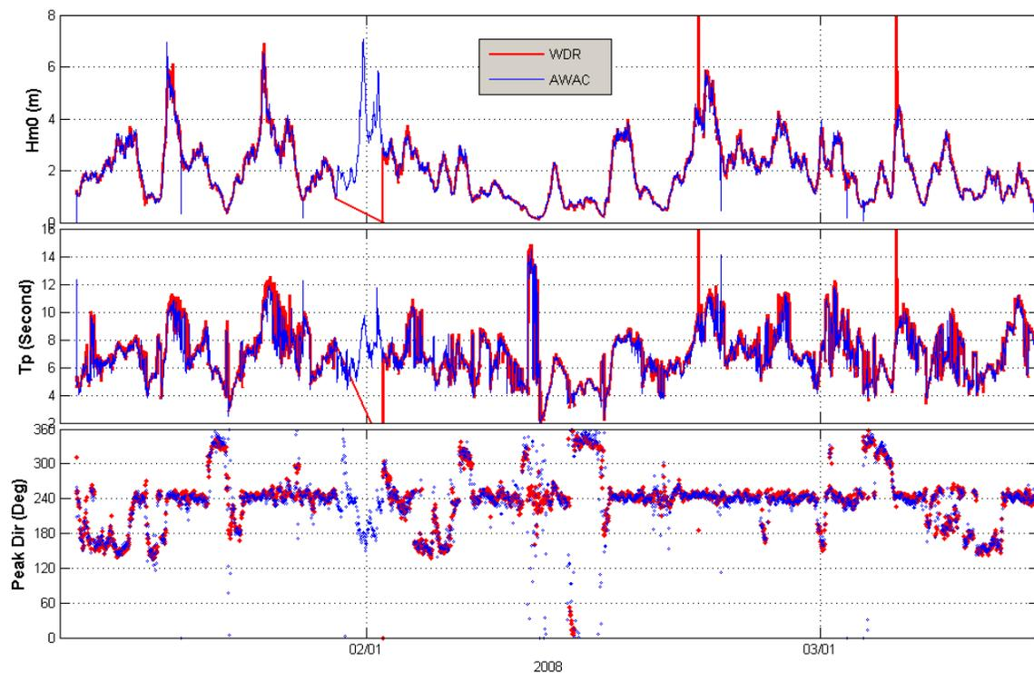
**Figure 7.** Wave estimates for the AWAC (blue) and Waverider (WDR - red). (a) Significant wave height, (b) Peak direction, (c) and peak direction.
