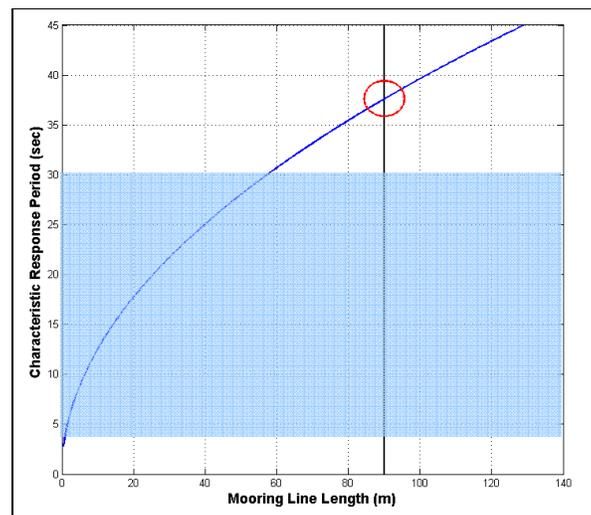
**Figure 5.** Characteristic response estimated for the SUBS buoy for a range of mooring lengths. The shaded region indicates the full range of the wave band that is desired to measure. The mooring at Lysekil was 90 meters long and as a result had a characteristic response of approximately 37 seconds (red circle); this is safely outside the wave band of interest.
