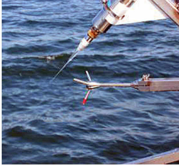
Figure 2. Detail photo showing Vector probe and fast-response O 2 sensor. The O 2 sensor is positioned to measure directly adjacent to the Vector sampling volume, 15 cm from the Vector probe.
