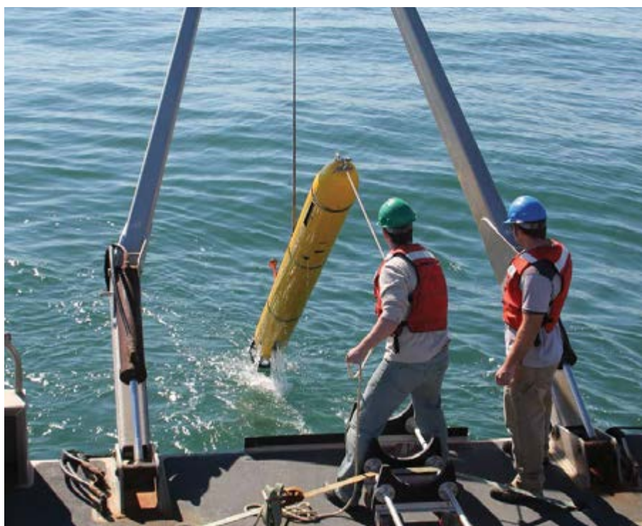
The Bluefin-12 AUV now carries the Solstice side-scan sonar from Sonardyne, which delivers images in high resolution. (Photo: Bluefin Robotics)
