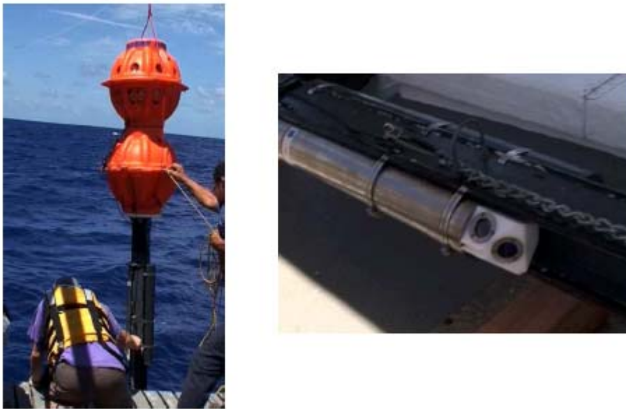
Fig.2 (left) Free-vehicle assembly from Apr 2008 deployment showing flotation spheres (orange); and Nortek Aquadopp current meter, counter-balance, and frame (dark gray). Ballast was suspended below the current meter assembly by 2 m steel chain (not shown). (right) Close up of Aquadopp transducer head and free-vehicle burn wire. Steel chain suspends ballast below free-vehicle (not shown). An identical burn-wire assembly is found on the other side of the ADCM frame and functions as a secondary, 'fail-safe' ballast release.
