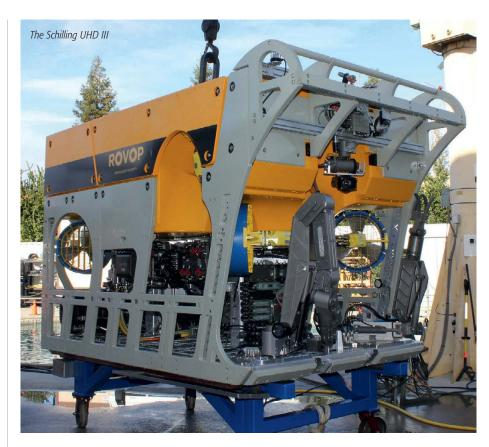
package can power a myriad of underwater tools for your mission needs too. Multiple gigabyte Ethernet options are available along with the hardware and software for underwater surveying, and surface weather monitoring. This midsize ROV can carry an impressive payload of 218 to 285 kilograms depending upon the buoyancy configuration. This ROV is transportable by air to any spot on the globe.
