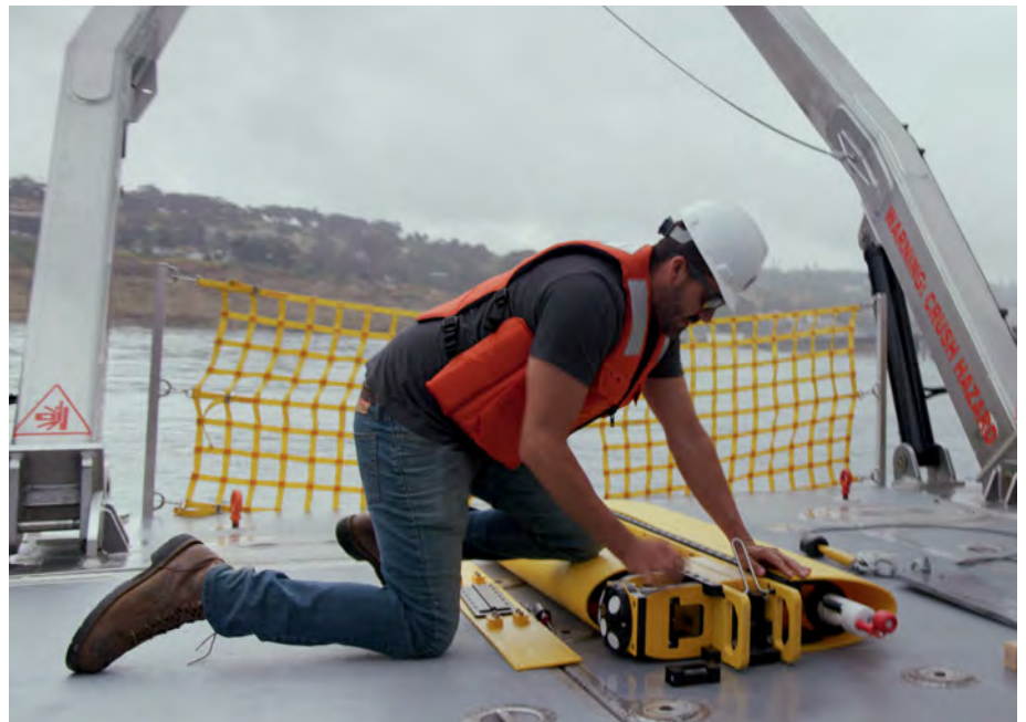
The Wirewalker can safely move instruments throughout the water column to collect data on the vertical ocean structure
