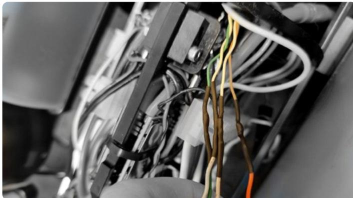
**10. Insert your connector in either port 2, 3 or 4 of the switch PCB.**
