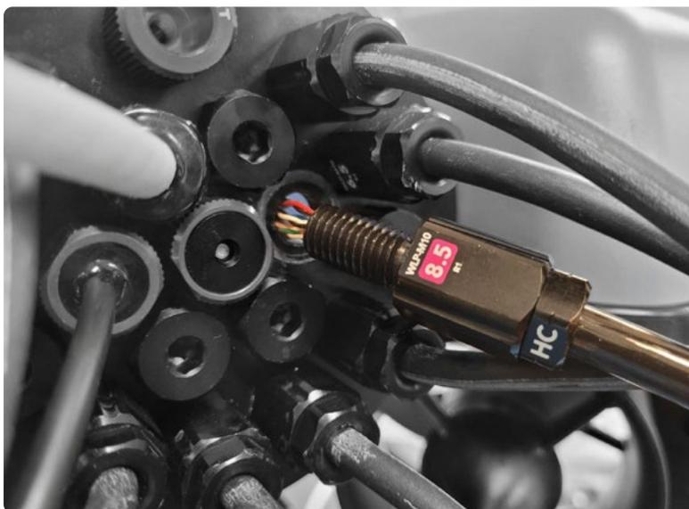
**8. Identify the Ethernet and Power wires. The other wires are for serial communication, and can be ignored/packed away safely (perhaps a shrink tube on the edge).**
