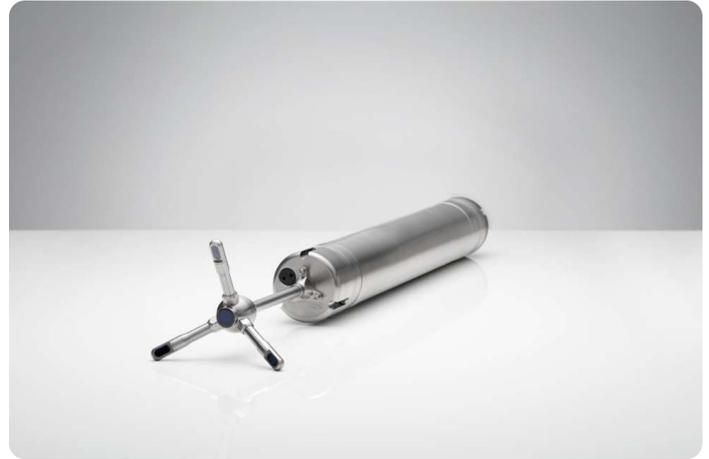
The Vector is a high-accuracy single-point current meter that is capable of acquiring 3D velocity in a very small volume at rates up to 64 Hz. It is widely used for sediment transport applications, small-scale turbulence measurements and coastal engineering studies. It has an excellent track record of delivering outstanding data quality in a variety of applications. This titanium version of the Vector is suitable for investigating deep-water currents down to depths of 4000 m.
