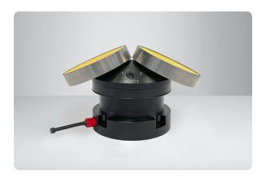
The 2D Horizontal Profiler is the ideal tool for current measurements from a physical structure in, for example, port entrances. This ADCP provides the two horizontal flow components at multiple distances from the mounting and is commonly used in online applications where immediate access to current data is critical.
