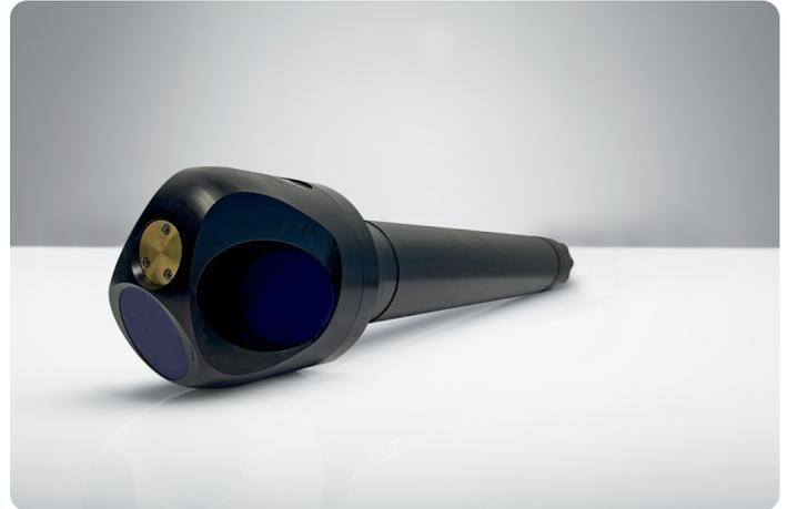
The Aquadopp Profiler is a highly versatile Acoustic Doppler Current Profiler (ADCP) available in four profiling range options, from < 1 m to > 85 m. The 600 kHz version has a current profiling range of up to 40 m. Designed for simple yet powerful operation, this current profiler is packed with features used by engineers and researchers to enable accurate and effective hydrodynamic data collection in a variety of environmental conditions.
