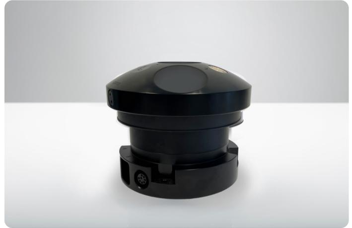
The AWAC 1 MHz ADCP has become the standard reference technology in submerged wave-measurement applications. Thousands of these ADCPs have been deployed to capture the full wave spectrum in combination with current profiles. With a 35 m maximum range for wave measurements, 4 Hz sampling of the surface elevation and onboard wave processing for real-time applications, the AWAC 1 MHz is the optimal tool for shallow current and wave measurements.
