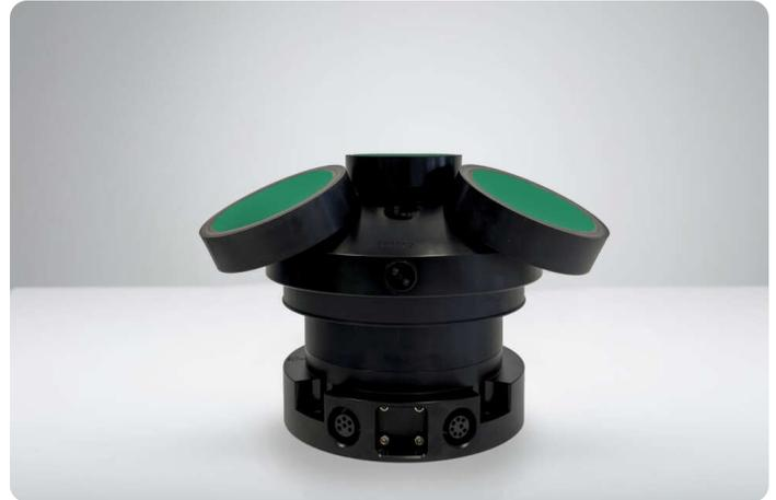
The AWAC 400 kHz ADCP has become the standard reference technology in submerged wave-measurement applications. Thousands of these ADCPs have been deployed to capture the full wave spectrum, in combination with current profiles. With a 100 m maximum range for wave measurements, 1.5 Hz sampling of the surface elevation and onboard wave processing for real-time applications, the AWAC 400 kHz is the optimal tool for deeper-water current and wave measurements.
