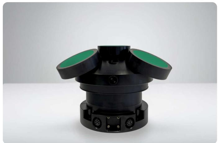
The AWAC 400 kHz ADCP has become the standard reference technology in submerged wave-measurement applications. Thousands of these ADCPs have been deployed to capture the full wave spectrum, in combination with current profiles. With a 100 m maximum range for wave measurements, 1.5 Hz sampling of the surface elevation and onboard wave processing for real-time applications, the AWAC 400 kHz is the optimal tool for deeper-water current and wave measurements.
