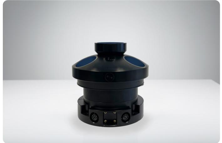
The AWAC 600 kHz ADCP has become the standard reference technology in submerged wave-measurement applications. Thousands of these ADCPs have been deployed to capture the full wave spectrum in combination with current profiles. With a 60 m maximum range for wave measurements, 2 Hz sampling of the surface elevation and onboard wave processing for real-time applications, the AWAC 600 kHz is the optimal tool for medium water-depth current and wave measurements.
