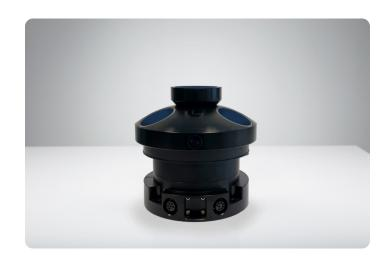
The AWAC 600 kHz ADCP has become the standard reference technology in submerged wave-measurement applications. Thousands of these ADCPs have been deployed to capture the full wave spectrum in combination with current profiles. With a 60 m maximum range for wave measurements, 2 Hz sampling of the surface elevation and onboard wave processing for real-time applications, the AWAC 600 kHz is the optimal tool for medium water-depth current and wave measurements.
