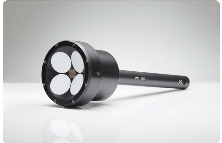
The DVL 333 Surface is a Doppler Velocity Log designed specifically for surface vessels. Traditional DVLs have a more vulnerable protruding head. The DVL 333 Surface mounts flush to the vehicle hull, alleviating this concern and minimizing drag and the risk of cavitation at the head.
