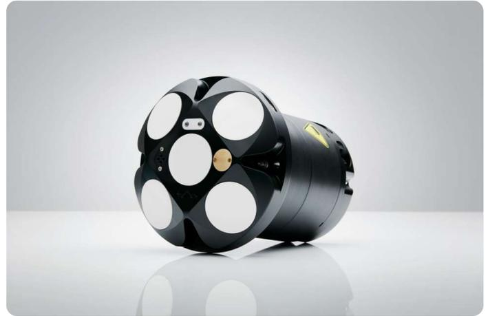
The Signature 500 ADCP is designed for flexibility. It measures current profiles at up to 8 Hz sampling frequency. It can also measure direct vertical velocity profiles, wave height and direction, and acoustic ranging to ice. The center beam also functions as a biological echosounder, enabling high-resolution measurements of biomass in the water column. All these features can be combined using Nortek’s patented concurrent mode technology.
