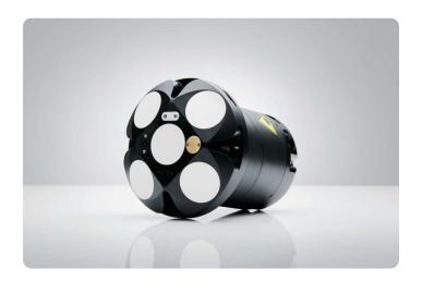
The Signature 500 ADCP is designed for flexibility. It measures current profiles at up to 8 Hz sampling frequency. It can also measure direct vertical velocity profiles, wave height and direction, and acoustic ranging to ice. The center beam also functions as a biological echosounder, enabling high-resolution measurements of biomass in the water column. All these features can be combined using Nortek's patented concurrent mode technology.
