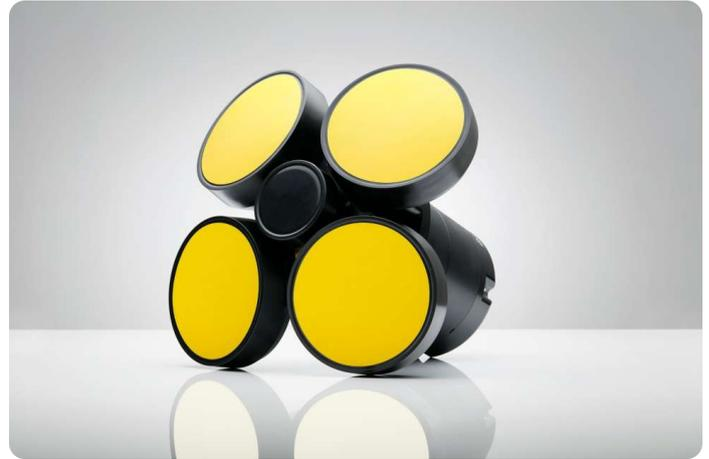
The Signature 250 ADCP is a medium-range current profiler with a suite of extra features. It has a current profiling range of 200 m, and can measure wave height, period and direction at depths as great as 150 m. The Signature 250 ADCP can also measure acoustic ranging to ice. Its compact design and low power consumption make it an ideal tool for long-term deployments in all waters.
