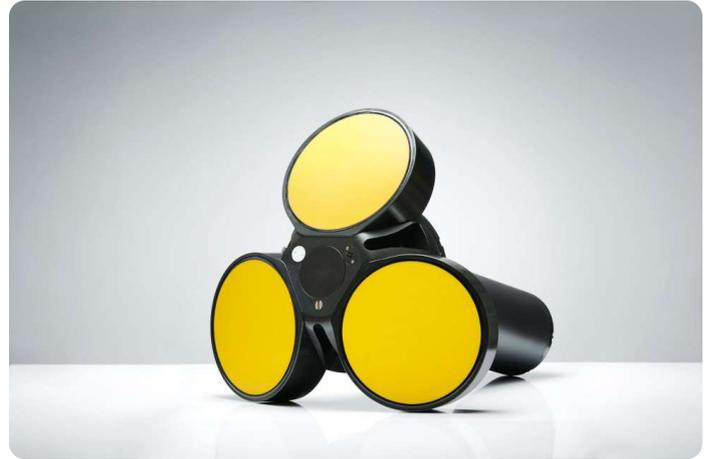
The Signature 55 ADCP is a current profiler that combines an ultralong range with a compact layout. Novel ADCP transducer design allows 1000 m profiles concurrent with slightly shorter-range, finer resolution measurements using two different frequencies in the same instrument. The more than 90% lower power consumption (compared to similar ADCPs) also permits long-duration deployments operating on internal batteries only.
