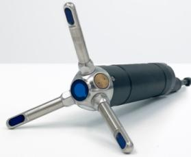
The Vector Generation 2 is a high-accuracy single-point current meter that is capable of acquiring 3D velocity in a very small volume at rates up to 64 Hz. It is widely used for sediment transport applications, small-scale turbulence measurements and coastal engineering studies. It has an excellent track record of delivering outstanding data quality in a variety of applications. This version is suitable for use down to a depth of 300 m.
