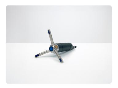
The Vector Generation 2 is a high-accuracy single-point current meter that is capable of acquiring 3D velocity in a very small volume at rates up to 64 Hz. It is widely used for sediment transport applications, small-scale turbulence measurements and coastal engineering studies. It has an excellent track record of delivering outstanding data quality in a variety of applications. This version is suitable for use down to a depth of 300 m.
